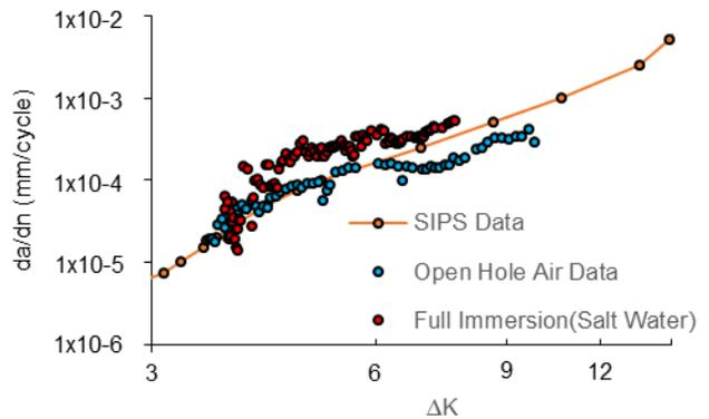
FIGURE 10. Fatigue crack growth rate data comparing laboratory air and full immersion in salt water
