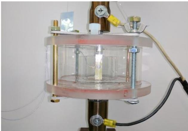
FIGURE 12. Open hole specimen in atmospheric test cell
