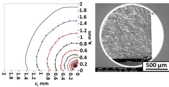
FIGURE 6. Example marker measurement and representative fracture surface
