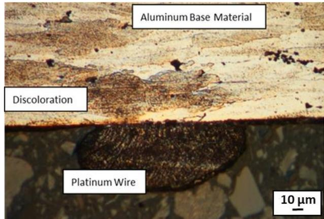
FIGURE 14. Micrograph of a cross-sectioned platinum spot-weld, discolored region indicating potential spot weld damage.
