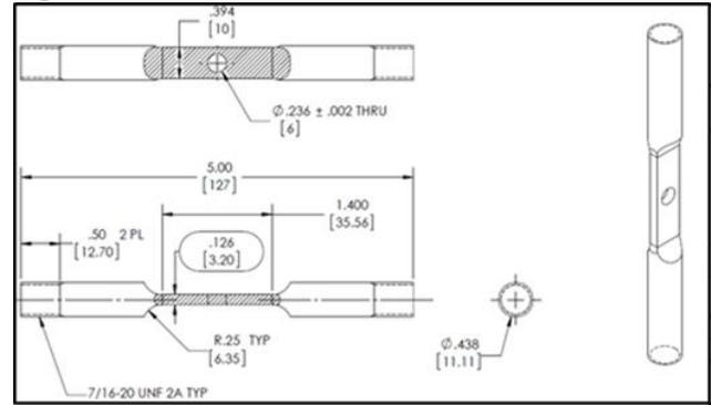
FIGURE 1. Typical Open Hole Specimen, inches [mm]
