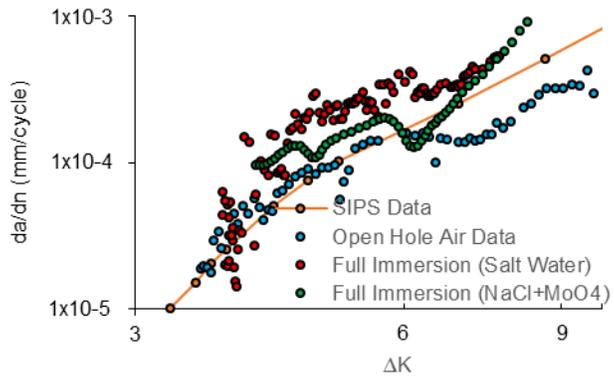
FIGURE 11. Comparison between laboratory air, full immersion in salt water, full immersion in salt water with added molybdate
