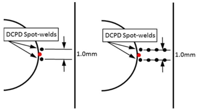
FIGURE 15. Schematic showing the standard DCPD spot-weld configuration vs. the stitched spot-weld configuration
