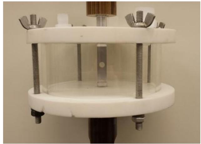
FIGURE 8. Open hole specimen installed in the full immersion test cell
