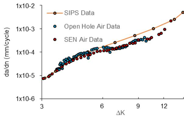
FIGURE 9. Crack growth rate comparison between characterized 7075-T651, open hole specimen, SEN specimen.
