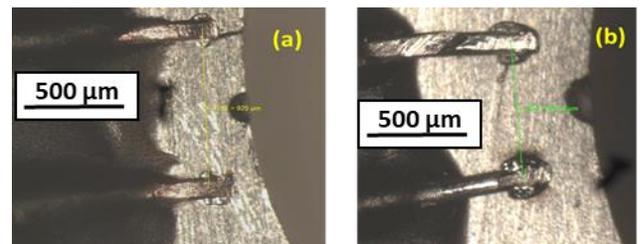
FIGURE 3. Typical arrangement of DCPD leads near laboratory created corrosion pits
