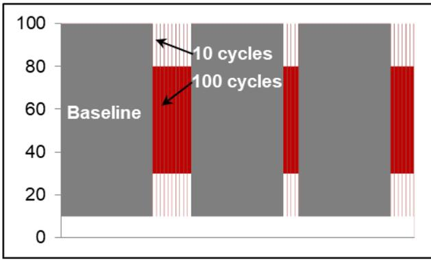
FIGURE 4. Schematic of applied marker spectrum
