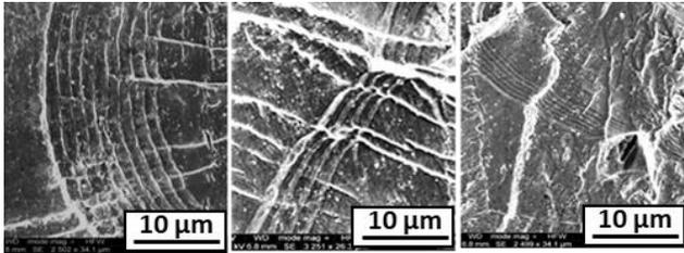
FIGURE 5. Scanning Electron Microscopy of marker bands as observed on the fracture surface
