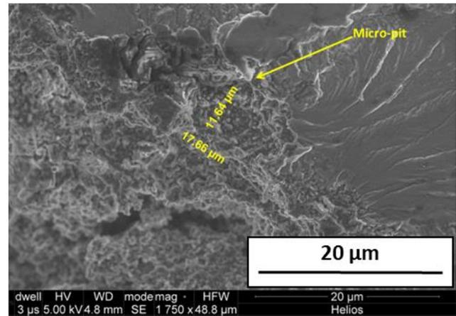
FIGURE 2. Scanning Electron Microscopy of micro-pit near the bulk material
