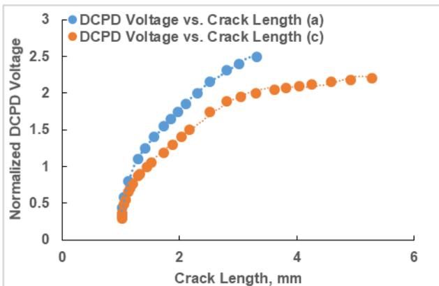
FIGURE 7. Calibration curve for normalized DCPD voltage and crack length
