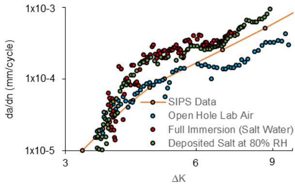
FIGURE 13. Comparison of fatigue crack growth rates between laboratory air and hydrated thin salt film test conditions.
