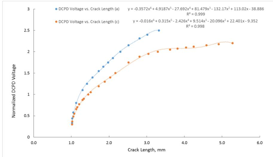
Figure 4. DCPD calibration curve for the open hole specimen.
