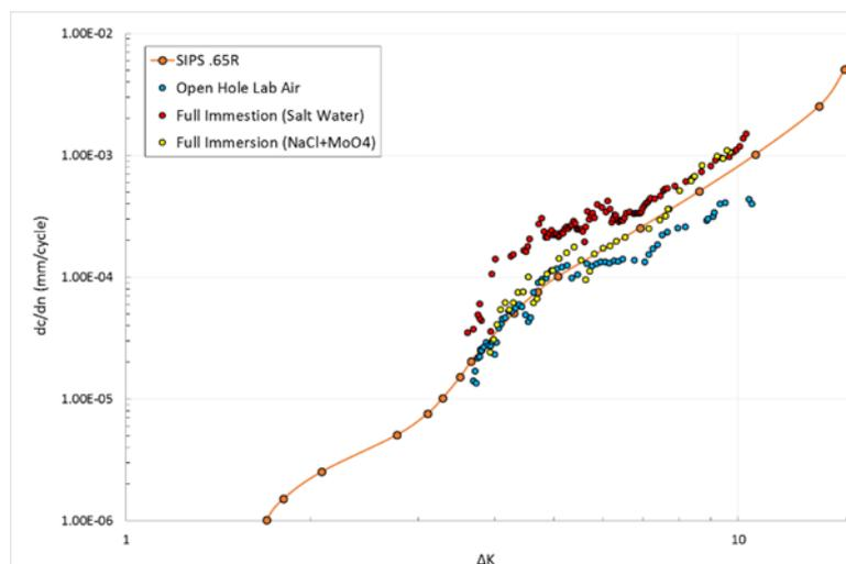
Figure 8. Comparison between laboratory air, full immersion in salt water, full immersion in salt water with added molybdate.
