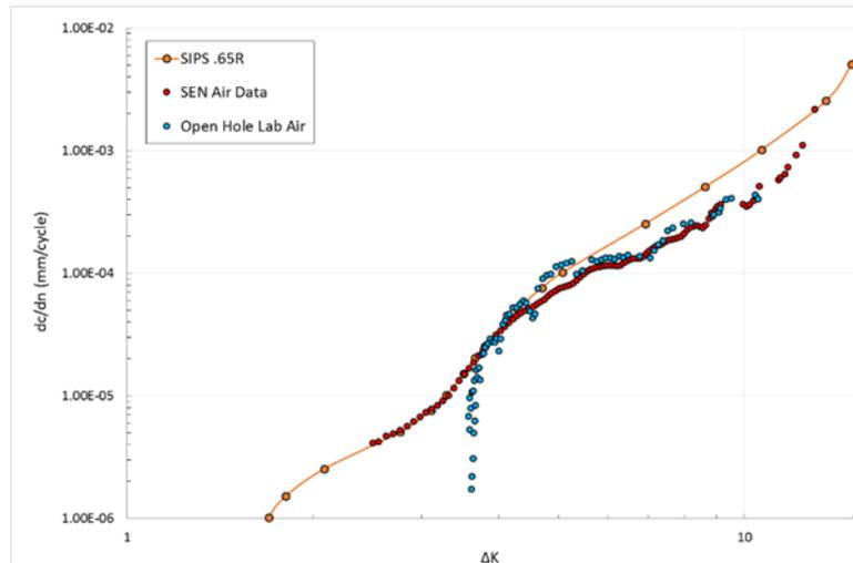
Figure 6. Crack growth rate comparison between characterized 7075-T651, open hole specimen, SEN specimen.
