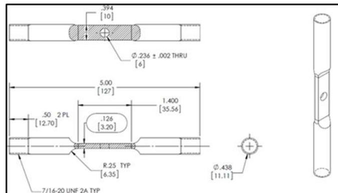
Figure 1. Open hole specimen geometry.
