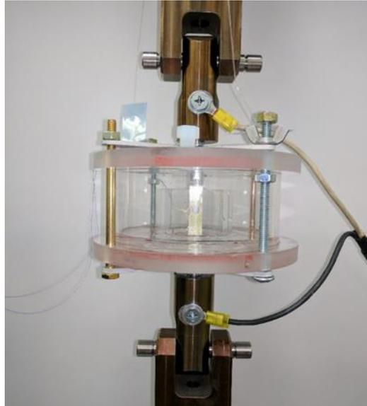
Figure 9. Open hole specimen in test cell.
