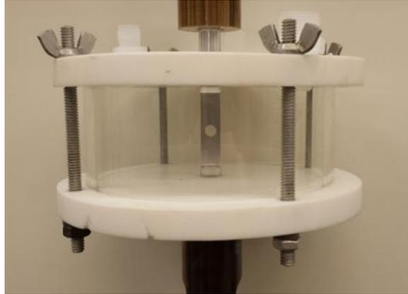
Figure 5. Open hole specimen in full immersion test cell.
