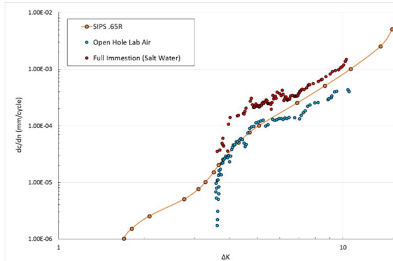
Figure 7. Fatigue crack growth rate data comparing laboratory air and full immersion in salt water.
