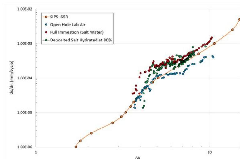
Figure 10. Comparison of fatigue crack growth rates between laboratory air and hydrated thin salt film test conditions.
