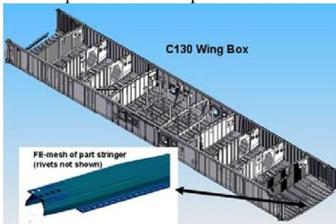
**Figure 1. C-130 CWB. Stringer shown exemplifies a characteristic mesh density**
