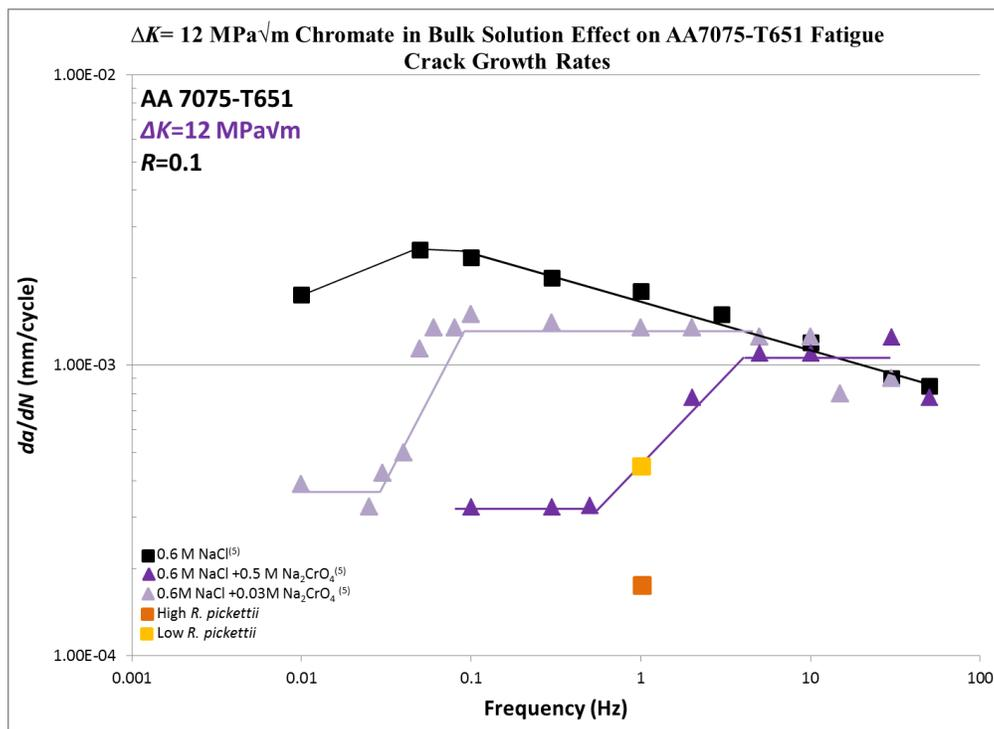
Figure 5: Comparison of the effect of *R. pickettii* on fatigue crack growth rates on AA7075-T651 to a known corrosion fatigue inhibitor chromate at  $\Delta K=12 \text{ MPa}\sqrt{\text{m}}$ ;  $R=0.1$ ,  $f=1 \text{ Hz}$  in  $0.6 \text{ M NaCl}$  <sup>(5)</sup>.
