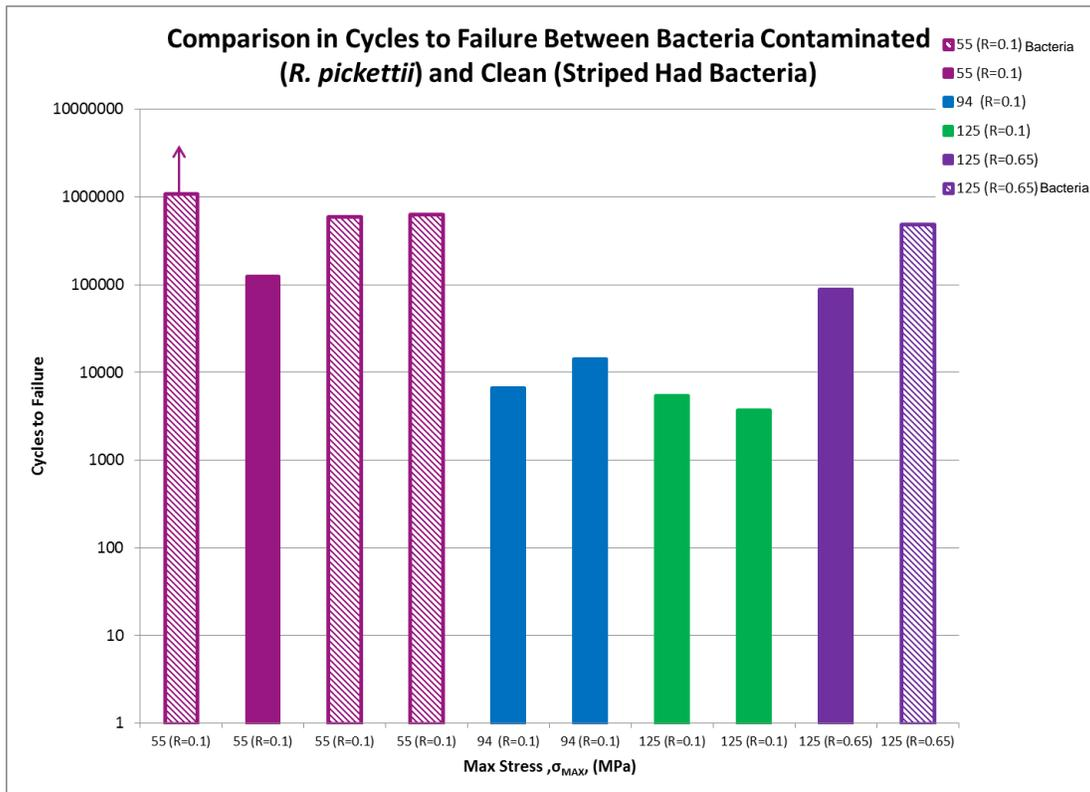
**Figure 3: Stress-life testing of *R. pickettii* compared to clean samples in 0.06M NaCl. The bacteria growth occurred randomly during testing, accounting for the fatigue tests completed without bacterial growth.**
