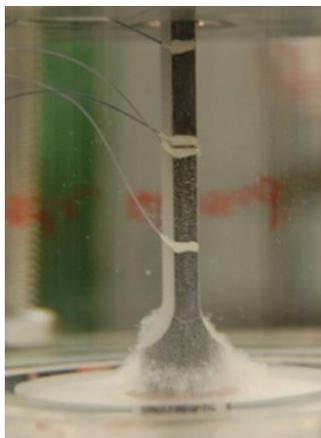
**Figure 2: Bacterial growth ("fuzz" at bottom of samples) on the 7xxx series aluminum alloy in 0.06M NaCl solution. The white on the dcPD wires is a protective coating. The fuzz continues up the entire length of the sample.**
