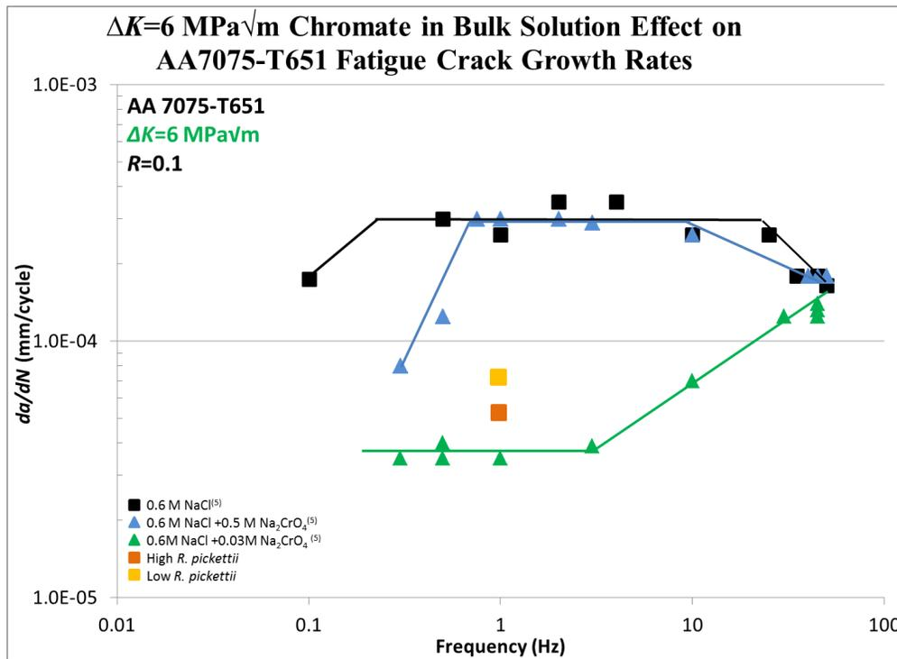
Figure 4: Comparison of the effect of *R. pickettii* on fatigue crack growth rates on AA7075-T651 to a known corrosion fatigue inhibitor chromate at  $\Delta K=6 \text{ MPa}\sqrt{\text{m}}$ ;  $R=0.1$ ,  $f=1 \text{ Hz}$  in  $0.6 \text{ M NaCl}$  <sup>(5)</sup>.
