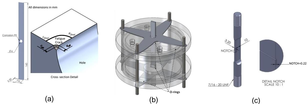
**Figure 1: (a) Fatigue sample with a preferential pit for crack initiation used in stress life corrosion fatigue testing. (b) Environmental test chamber used for corrosion fatigue testing. (c) Single edge notch (SEN) specimens were made of 7xxx series aluminum alloy. All dimensions are in millimeters (mm).**
