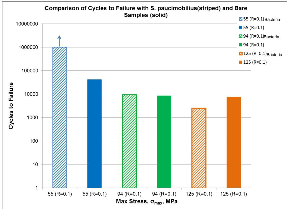
Figure 7: Stress-life testing of *S. paucimobilis* compared to clean tests. Arrow denotes test did not fail after 1,000,000 cycles.
