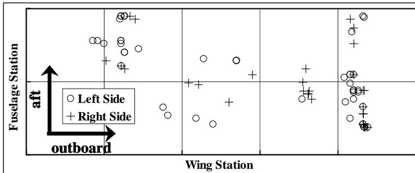
**Figure 9: Wing station (WS) and fuselage station (FS) location of all operational usage damage findings in the center wing of the category B aircraft teardown program.**
