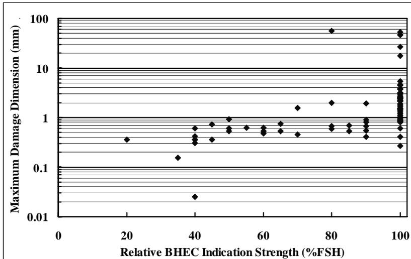
**Figure 3: Maximum fatigue crack damage dimensions as a function of eddy current indication in %FSH.**
