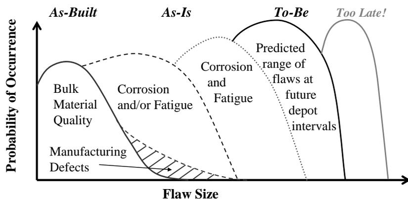
**Figure 11: Comparison of various IDS dimensions from C. Brooks 1999 ASIP Conference presentation titled “Correlation of Life Prediction Methods with Corrosion-Related Tests”**
