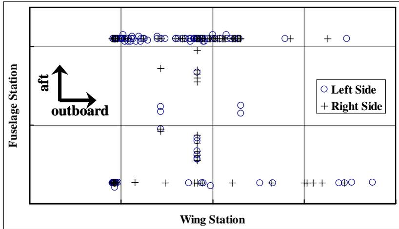
**Figure 10: Wing station (WS) and fuselage station (FS) location of all operational usage damage findings in the wing of all category A aircraft teardown programs.**
