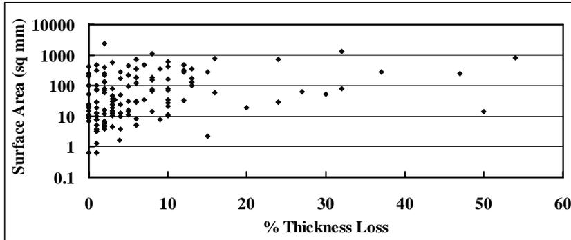
**Figure 7: Percentage of maximum part thickness lost due to surface corrosion damage plotted against the total surface area affected at the evaluated site.**
