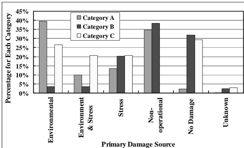
**Figure 2: Damage finding types for all teardown programs broken out by aircraft category.**
