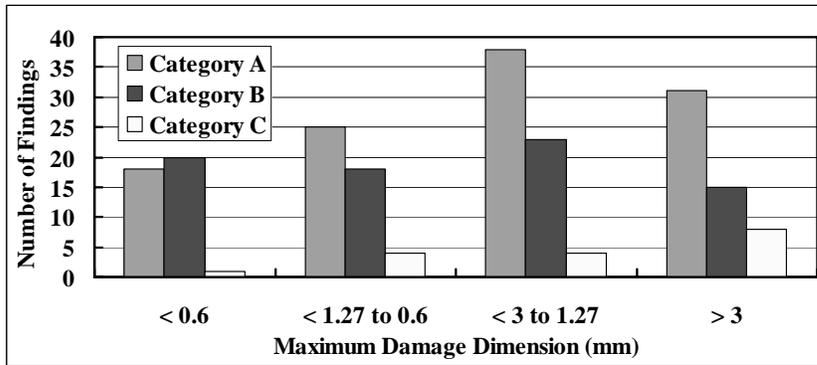
**Figure 6: Histogram of maximum damage dimension for all operational usage damage cracks characterized in the subject teardown programs broken out by aircraft category.**
