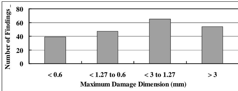
Figure 4: Histogram of the maximum damage dimension for all operational usage crack damage characterized in the subject teardown programs.
