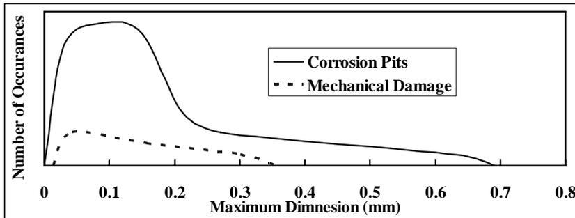
**Figure 8: Distributions of measured initiation features by feature type.**
