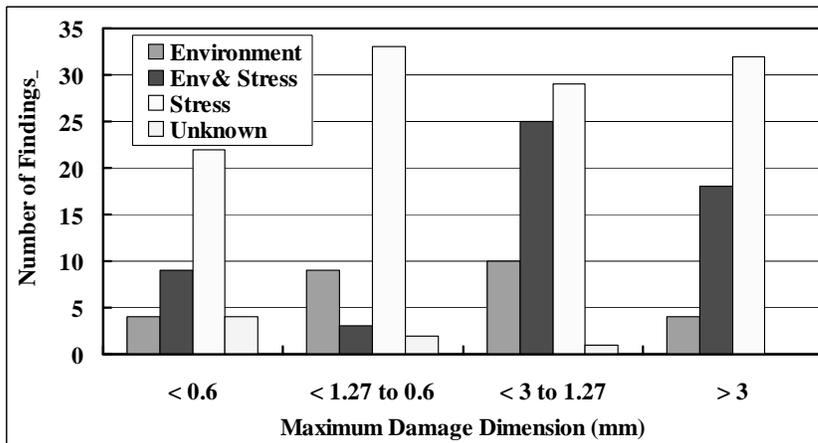
Figure 5: Histogram of maximum damage dimension for all operational usage damage cracks characterized in the subject teardown programs broken out by primary damage source.
