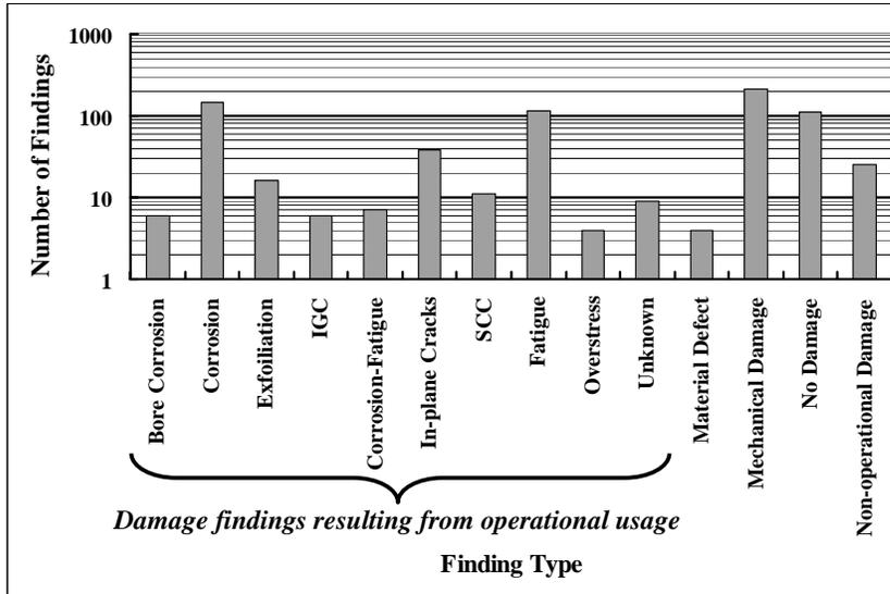
**Figure 1: Damage finding types for all teardown analysis programs.**
