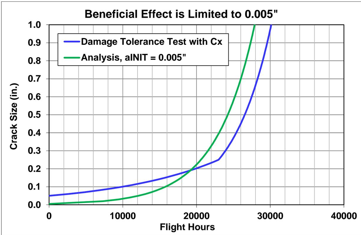
Figure 1. Beneficial Effect is Limited to Initial Crack Size = 0.005 inch
