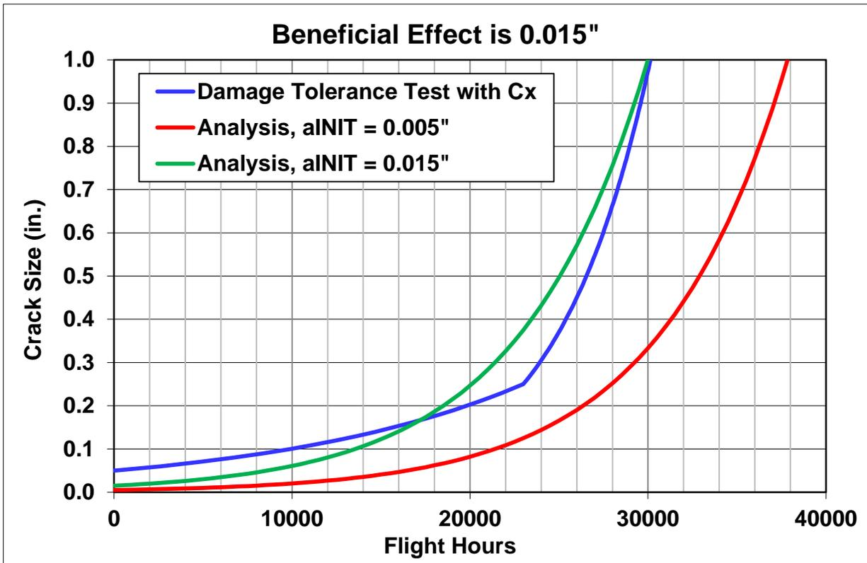
Figure 2. Beneficial Effect Requires Use of Initial Crack Size > 0.005 inch
