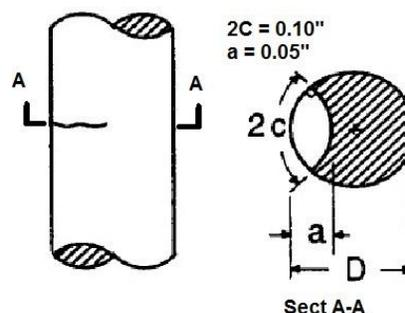
Figure 1: Revised Initial Flaw Size for Pins and Fasteners
