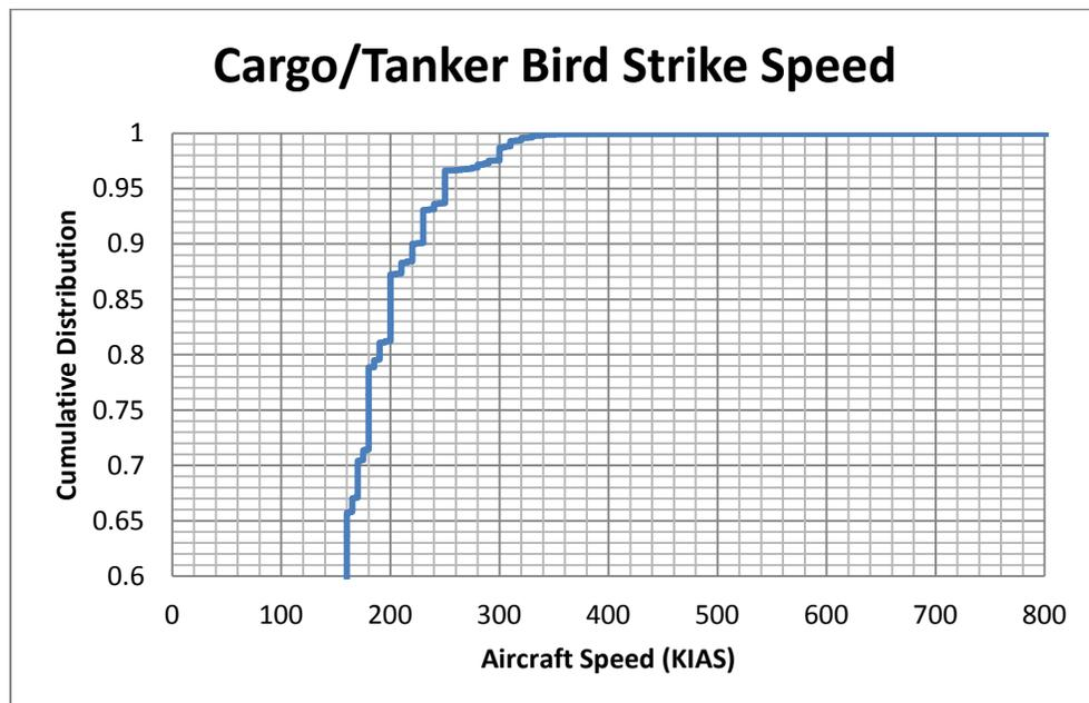
Figure 4 - Bird Strike Speed for Cargo/Tanker Aircraft
