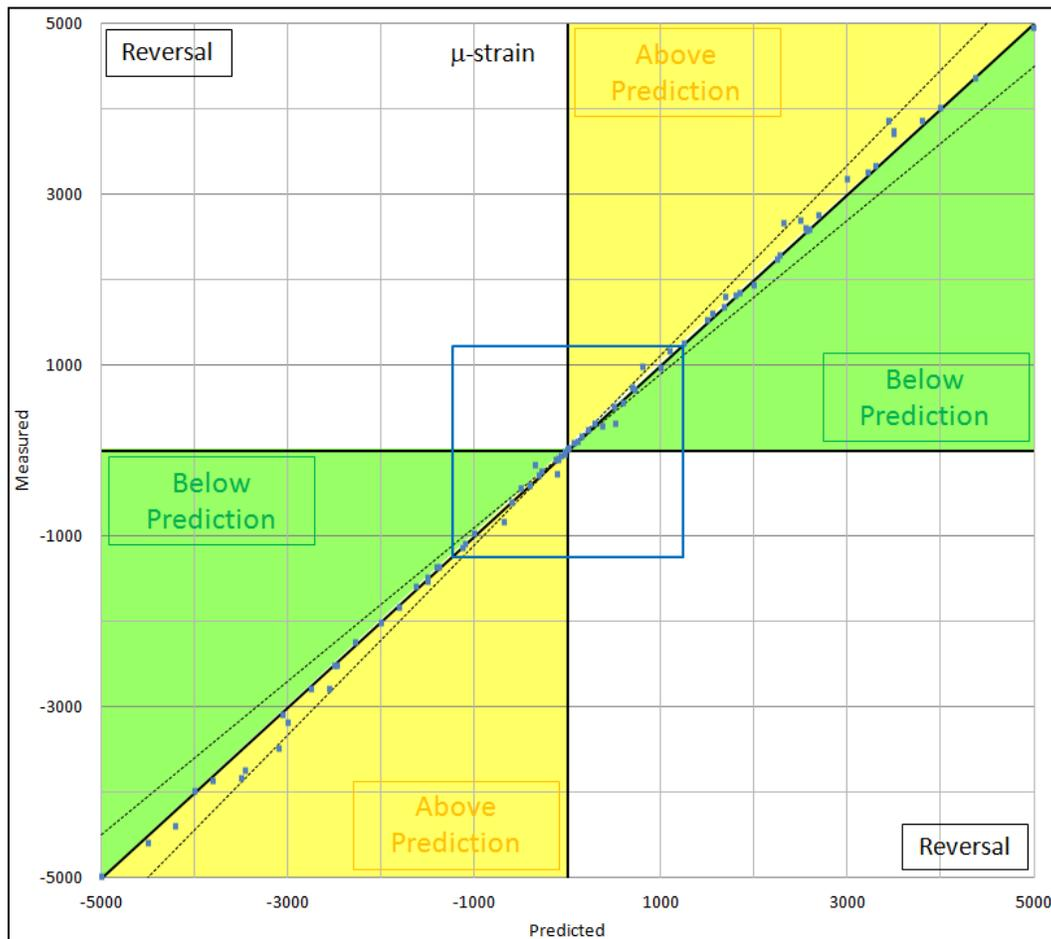
**Figure 3** – Sample Correlation Plot with Strain Threshold Box for the Material
