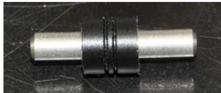
Figure 3. Wire-spacing pulley with 1 mm spacing between grooves.
