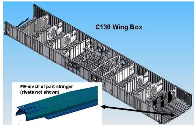
Figure 4. Center C-130 wing box which currently is being meshed in large detail at USAFA. Stringer shown in the figure exemplifies a characteristic mesh density.
