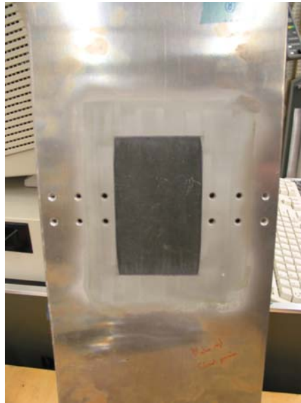
Figure 7: Boron-epoxy repair after bonding
