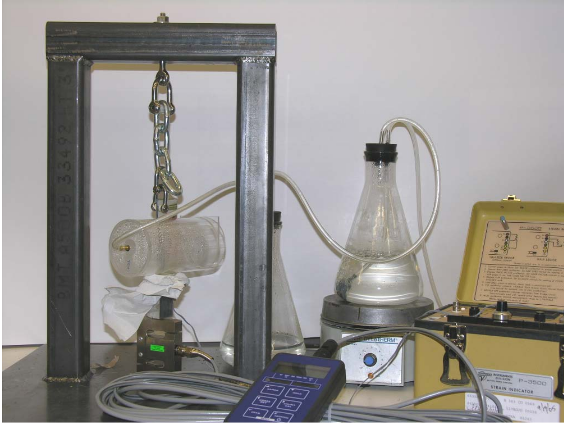
Figure 7. Constant displacement load frame with DI water fog environment.
