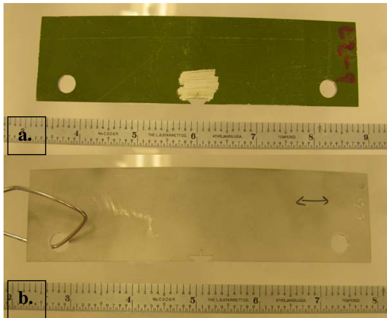
Figure 5. Coated and uncoated samples. Figure "a," above, has chromate coating covering the surface except for the machined edges of the part and the notched portion of the sample, where coating removal was necessary to machine the notch with EDM. Figure "b" was soaked in acetone to soften the coating, then scraped clean before final machining.
