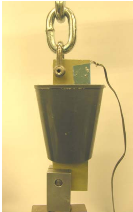
Figure 8. Specimen tested with cup in place for bath. Strain gage wire is also visible. No grips are immersed in the bath.
